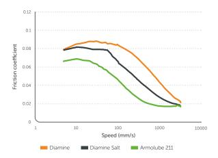
Addition of 0.5 wt% of Armolube 211 in base oil including ZDDP. MTM test at  $120^{\circ}$ C and 50/50 slide roll ratio.
