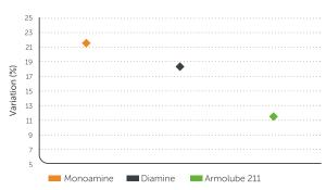
Volume change in seals testing, addition of 1.0 wt% of Armolube 211 in base oil for 1 week at 150°C.
